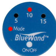
Diagram 2: LEDs indicating 10 second ramp mode.
